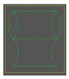
This die-board layout in SteelRules allows one click output to a laser or router.
